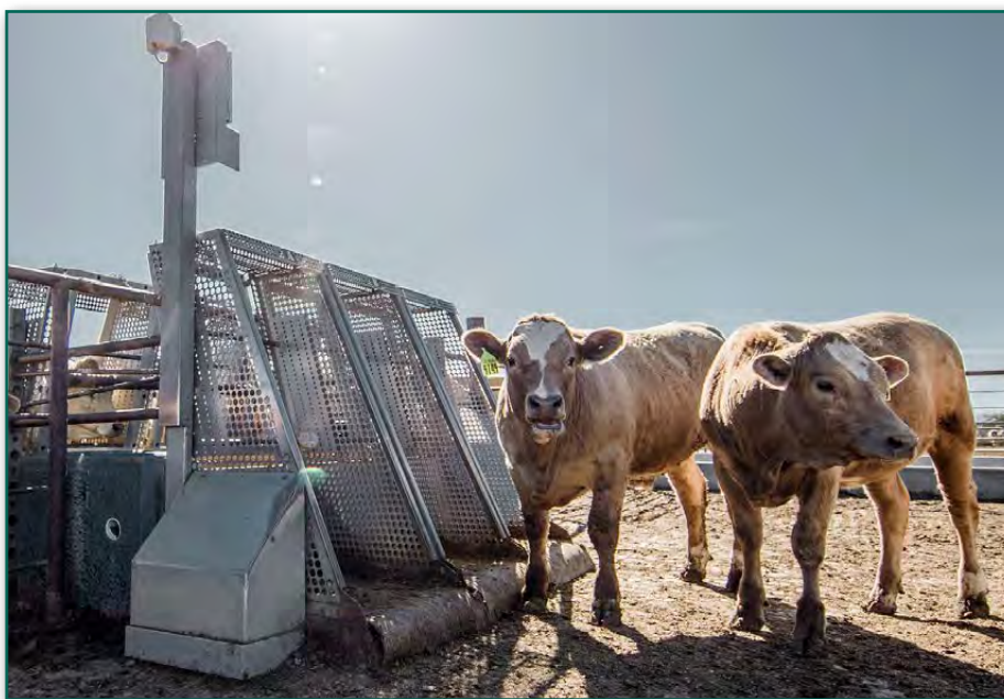
Photo 1: A weighing platform conjoined with a water trough to weigh the front half of an animal multiple times per second as it drinks. An electronic ID tag links the animal to the weights that are captured
