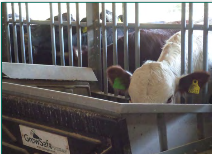
Photo 2: The GrowSafe feed bunker stand on weighing cells so that feed intake can be measured. The animals have electronic tags and the animal that eats is identified and also how much it ate. In this way, feed intake of individual animals that are in a group can be measured
